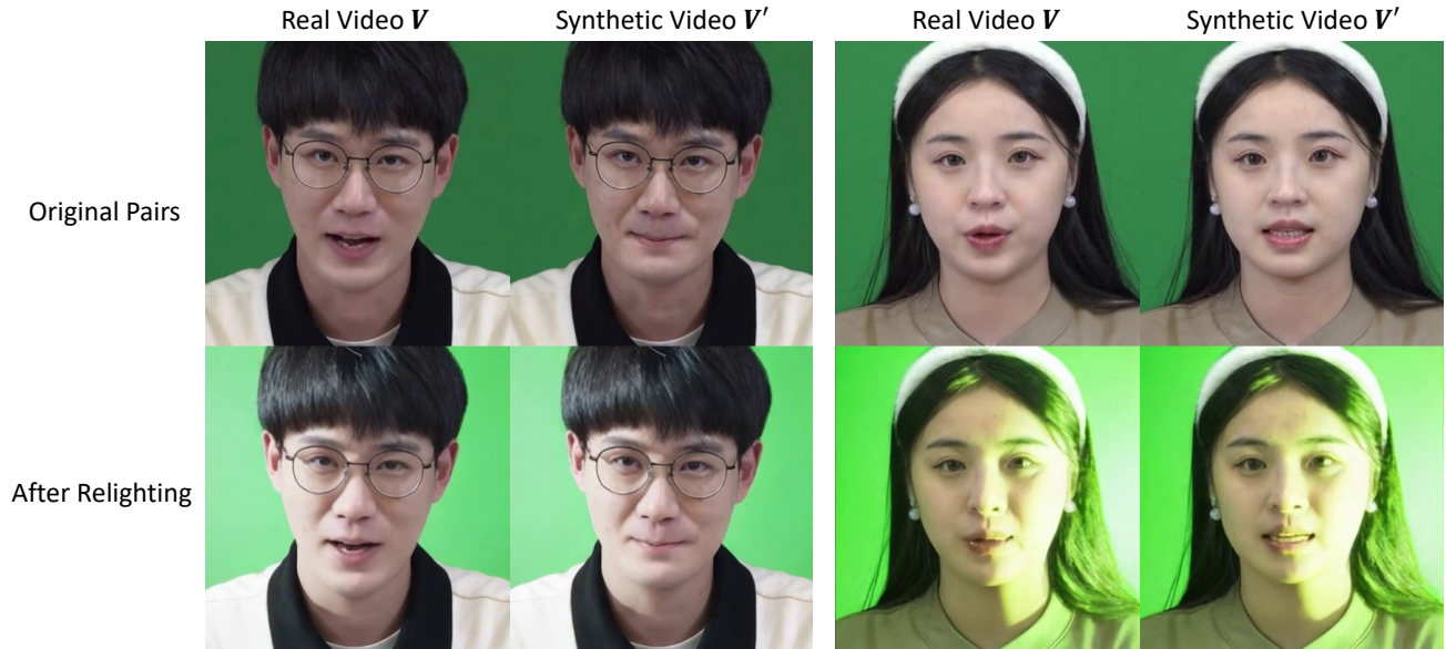
Figure 8. Visualizing the lighting augmentation strategy. We apply identical static and dynamic relighting effects (e.g., changing color, intensity, and direction) to both the generated contextual reference and the target video. This ensures the mask-free video dubber learns to utilize lighting cues from the complete input video even under varying illumination conditions.
