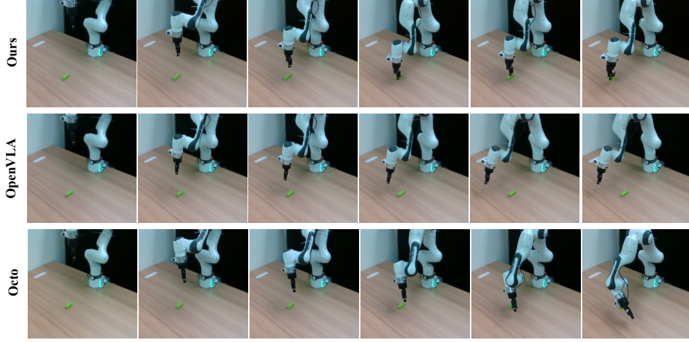
Figure 1: Visualization of zero-shot generalization of different models. The first row is Diffusion Transformer Policy(ours). The second row of demonstration is OpenVLA Kim et al. (2024), the third row is Octo Team et al. (2024). Our Model can complete the tasks successfully while both of the others fails.
