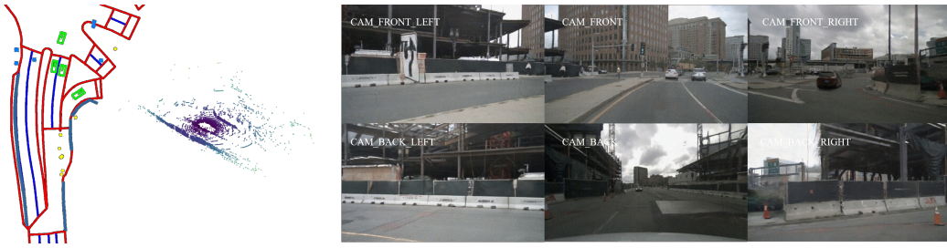
Figure 6: Joint generation of LiDAR and multi-view video. Our method generates spatially aligned LiDAR and camera views conditioned on a Busy junction layout.
