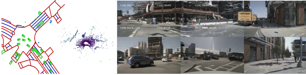
Figure 7: Joint generation of LiDAR and multi-view video. Our method generates spatially aligned LiDAR and camera views conditioned on a turning layout.
