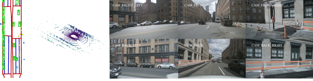
Figure 5: Joint generation of LiDAR and multi-view video. Our method generates spatially aligned LiDAR and camera views conditioned on a shared straight street layout.
