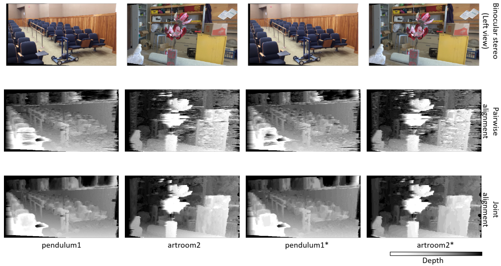
Figure S6: Results of extracting depth information. The top row, second row, and the last row show the left view of binocular stereo, pairwise alignment result, and joint alignment result.
