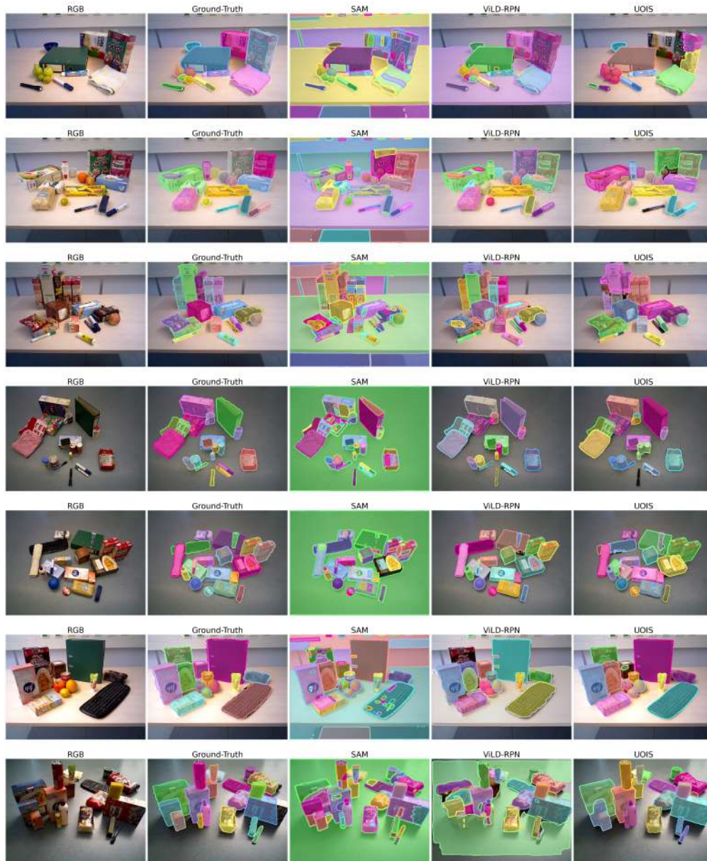
Figure 6: Comparison of different segmentation models for seven example cluttered indoor scenes from OCID dataset
