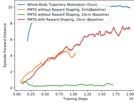
Figure E.3: PMTG does not learn to trot across 10cm gaps without shaped reward. Our method with whole-body low-level controller converges rapidly without shaped reward for gap crossing.
