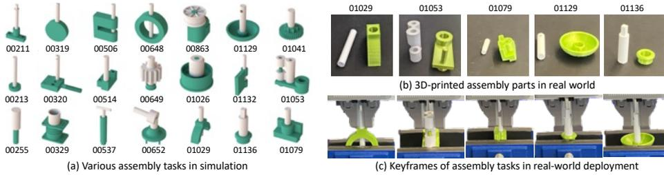
Figure 2: **Illustration of assembly tasks in AutoMate and SRSA.** (a) Samples of assembly tasks in the AutoMate benchmark. (b) 3D-printed parts of corresponding real-world assembly tasks in SRSA. (c) Keyframes from video recordings of our real-world deployments of performant policies.
