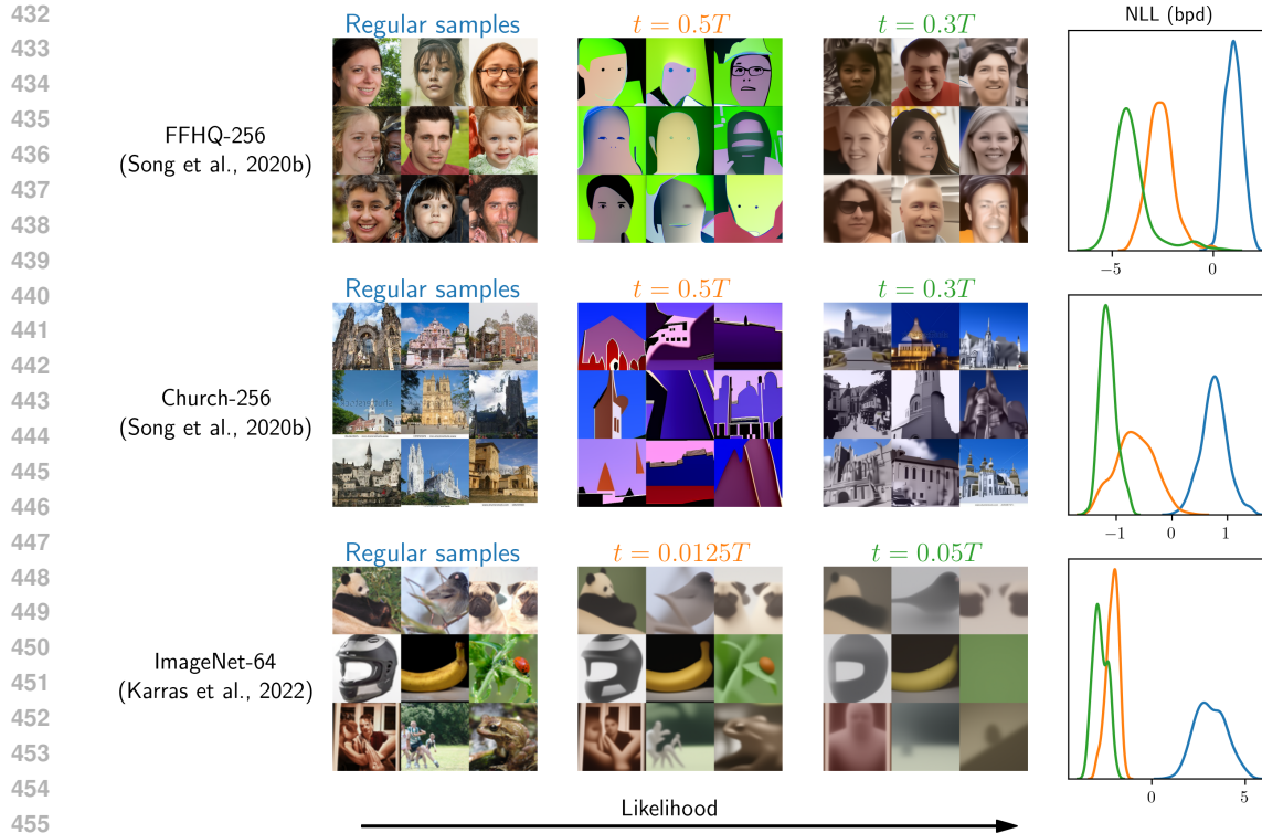
Figure 9: Diffusion models assign highest likelihoods to unrealistic images. Left: High-density samples generated with Algorithm 1 for various values of the threshold parameter t . Right: distributions of negative log-likelihood (in bits-per-dim). Across different models and datasets, Algorithm 1 finds unnatural images, which have higher densities than regular samples.
