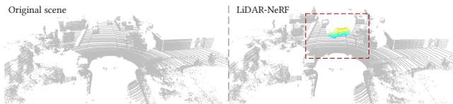
**Figure 9: Scene editing. The augmented scene from our LiDAR-NeRF has realistic occlusion effects and consistent LiDAR pattern.**
