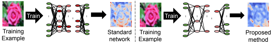
Figure 1: Concept: We consider a novel problem of distortion in latent features of a network in the presence of adversarial perturbation, where the model observes different degrees of distortion for different features (brighter red indicates higher level of distortion). To solve this problem, our proposed method learns a bayesian pruning mask to suppress the higher distorted features in order to maximize it’s robustness on adversarial perturbations.
