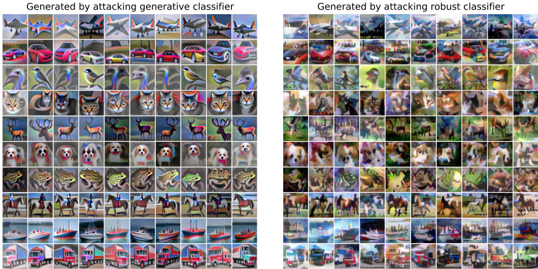
Figure 6: Images generated from class-conditional Gaussian noise by performing targeted attack against the generative classifier and robust classifier. we use PGD attack of steps 60 and step-size 0.5 \times 255 to perform L_2 \epsilon = 30 \times 255 constrained attack (same as Santurkar et al. (2019)). The Gaussian noise inputs from which these two plots are generated are the same. Samples not selected.
