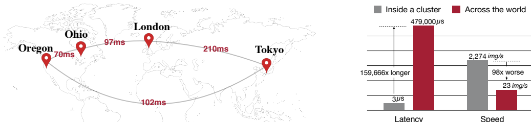
Figure 2: Network conditions across different continents (Left) and the comparison between connections inside a cluster (Right). Different from training inside a data center, long-distance distributed training suffers from a high-latency network, which proposes a severe challenge to scale across the world.
