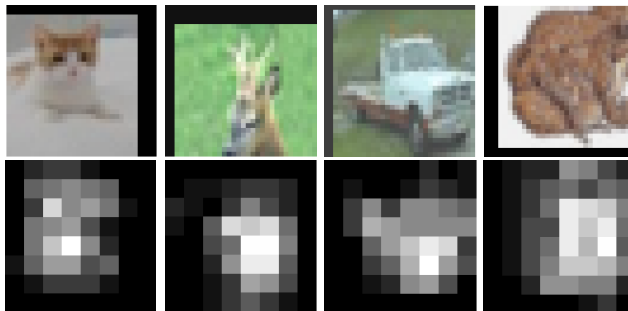
Figure 5: Visualization of gating probability – Top: feature maps from the final precision gating block in ResNet-18 on CIFAR-10. Bottom: probability of computing in high-precision (brighter pixel means higher probability). PG effectively identifies the location of the object of interest and increases bitwidth when computing in this region.
