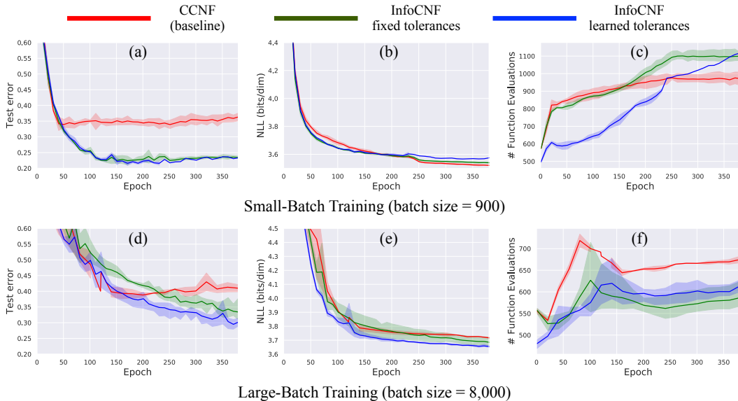
Figure 3: Evolution of test errors, test NLLs, and NFEs from the ODE solvers during the training of InfoCNF with learned tolerances vs. InfoCNF with fixed tolerances vs. CCNF (baseline) on CIFAR10 using small batch size (top) and large batch size (bottom). Each experiment is averaged over 3 runs.
