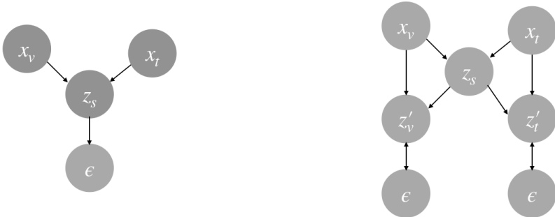
Figure 5. Inference model of our approach in comparison to conditional variational autoencoder of AG-CVAE (Wang et al. (2017)). AG-CVAE models only supervised information in the latent dimensions. Our model encodes domain-specific variations in the conditional priors z'_v and z'_t .
