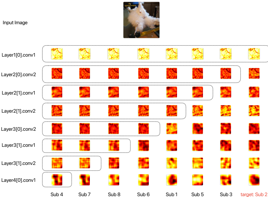
Figure 4: Visualization of Split-Ensemble’s learned features using Score-CAM. The number of splits is set to 8 and the model is trained on ImageNet1K with ResNet-18 as backbone. The feature maps within the dashed lines across the layers indicate shared representations. The input image’s class is ‘Angora’, targeted by submodel 2.
