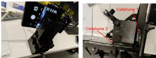
Figure 6: The real photos of our hardware. We use two OPPO Find X6 cellphones to build the hardware.
