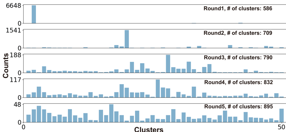
Figure 6: Clusters generated by DBSCAN over training rounds. The results of the first 5 rounds are shown. For the convenience of visualization, we only display 50 clusters and the number of data points in each of them.
