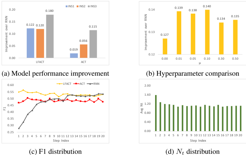
Figure 2: Results of RNN based models. (a) F1 score improvements over RNN on financial data set three instances (INS1, INS2 and INS3). (b) Average F1 improvements over RNN for different \mu values on all three instances. (c) Average F1 score at each step on INS1. (d) Average computation time ( N_t ) for LFACT on INS1.
