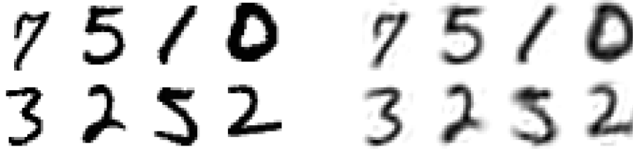
Figure 19: left : original MNIST handwritten digits, right : MNIST handwritten digits projected on the fifty principal components.
