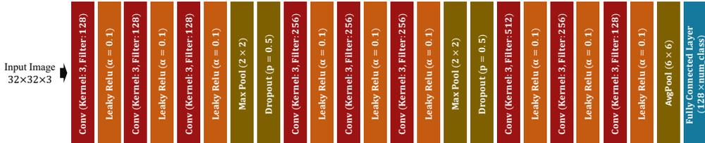
Figure 4: Illustration of the 13-layer Convolutional Network.
