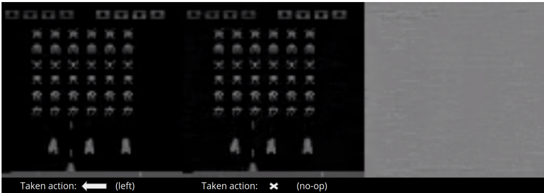
Figure 6: DQN playing Space Invaders. On the left, the unattacked current observation. In the middle, a mask of CopyCAT is applied to lure the agent into taking the "no-op" action. Parameters used are: \epsilon = 3 \cdot 10^{-2} , \alpha = 1.3 \cdot 10^{-5} . The L_2 norm of the corresponding mask (shown on the right) is 0.78. For this same \epsilon , FGSM- L_\infty would produce an attack of L_2 norm: 2.52
