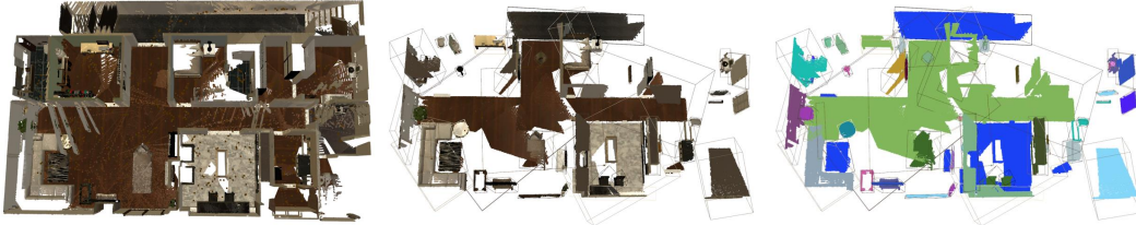
Figure 11: ConceptGraph pipeline. Left to right: Point-cloud of the scene built from a trajectory; All objects detected by ConceptGraphs pipeline after assigning a category-name based on CLIP; Semantic visualization of the apartment with color-coded class categories per furniture
