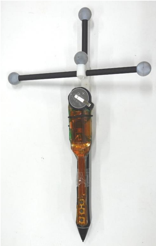
Wacom pen with custom mount bearing tracking markers and Bluetooth shutter button
