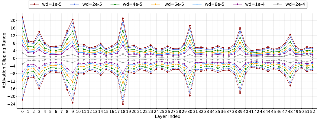
Figure 13: Activation clipping range learned by LSQ, given different L_2 regularization of the scale parameter.
