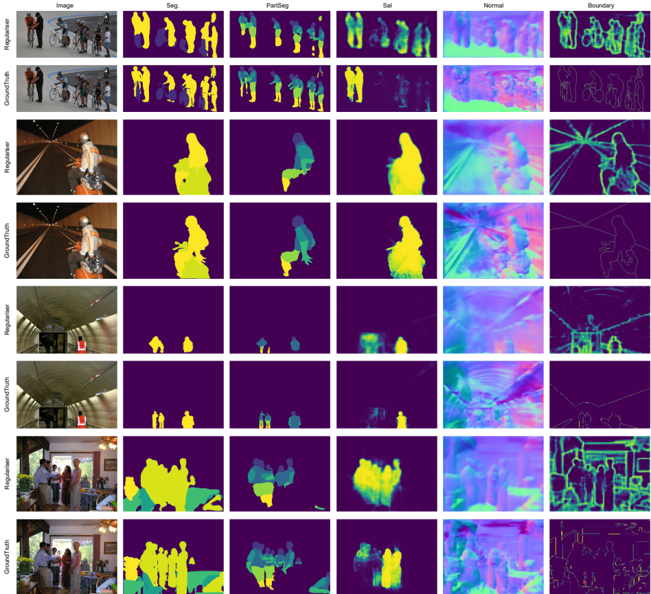
Figure 1: Qualitative results on PASCAL. Each column shows the image or predictions of our method’s regularizer branch or the groundtruth for each task, respectively.
