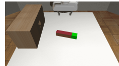
Peg Insertion: the robot must pick up the peg and insert it into the opening of a wooden block.
