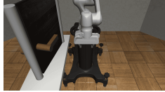
Door Opening: the robot must turn the door handle and open the door.
