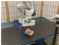
Stack: the robot must pick up the butter box and stack it on top of the popcorn box.
