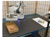
Cleanup: the robot must (1) pick up the butter box and place it into the bin and (2) push the popcorn to the right side of the table (the white area).
