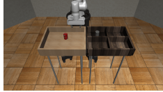
Pick and Place: the robot must pick up a soda can and place it into a specific target compartment.
