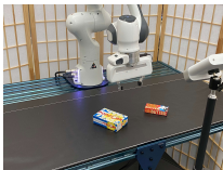
Stack: the robot must pick up the butter box and stack it on top of the popcorn box.
