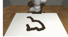
Wipe: the robot must wipe a table containing spilled debris. A penalty is given if the robot presses too hard into the table.
