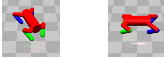
Figure 14: doggo robot: a quadrupedal robot with bilateral symmetry with 12-dimensional control space.
