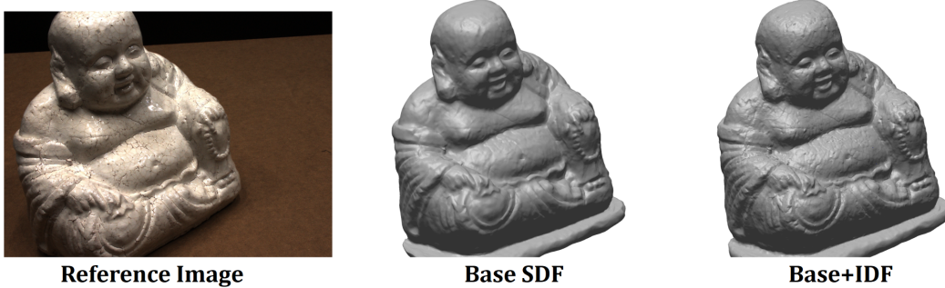
Figure 12: The visualization of the SDF decomposition. The left is the referene image, the middle is base SDF, the right is the combined SDF.
