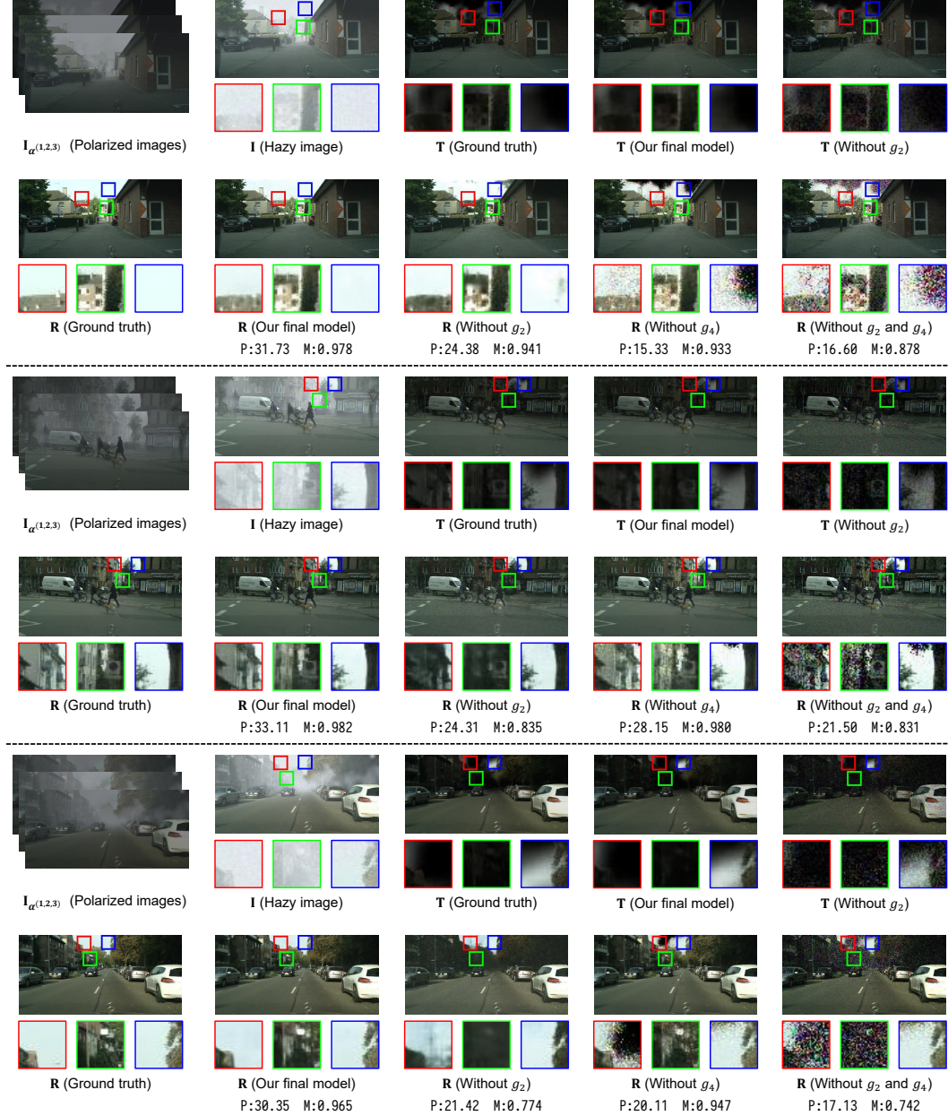
Figure 11: Qualitative comparisons on synthetic data without refinement (including the transmitted light \mathbf{T} and the original scene radiance \mathbf{R} ). Quantitative results evaluated using PSNR (P) and MS-SSIM (M) are displayed below each image.
