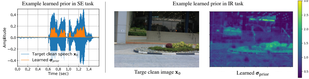
Figure 3: Visualizing the prior distribution learned by RestoreGrad. Here, the assumed form of the prior is a Gaussian: p_{\psi}(\epsilon|\mathbf{y}) := \mathcal{N}(\epsilon; \mathbf{0}, \text{diag}\{\sigma_{\text{prior}}^2(\mathbf{y}; \psi)\}) , where \sigma_{\text{prior}} is estimated by the neural network \psi with input \mathbf{y} . It appears that \sigma_{\text{prior}} follows the level variation of the speech waveform and preserves the structure of the original image. This indicates that an informative prior approximating the data distribution has been obtained for improved efficiency of the diffusion process.
