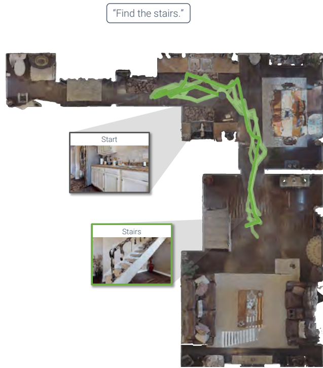
Figure 4: Qualitative example of successful navigation to the “ stairs .” The number of steps taken by our agent over five trials ranges from 80 to 102.
