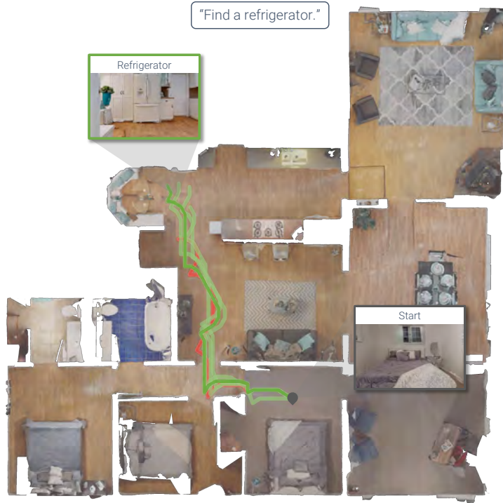
Figure 7: Qualitative example of “Find a refrigerator.” The agent succeeds in 4 of 5 trials (green) from the same starting position. In the failure (red) the agent stop short of fridge. The number of steps ranges from 83 to 99.
