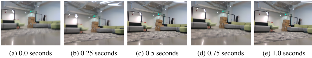
Figure 6: Quick motions and large changes in rotation occurring over one second. These quick motions cause degraded image captures on the quadraped affecting the deployment of the visual baseline. Changes in pitch (Fig. 6a,6b,6c,6d,6e) and roll (Fig. 6a and Fig. 6e) are notable.
