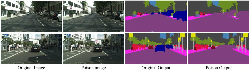
Figure 4: Visualization of images and models’ predictions on them. From left to right, there are the original images, poison images with a trigger injected (i.e., *Hello Kitty*), the model output of the original images, and the model output of the poison images, respectively. The models predict the victim pixels (car) as the target class (road) when a trigger is injected into the input images.
