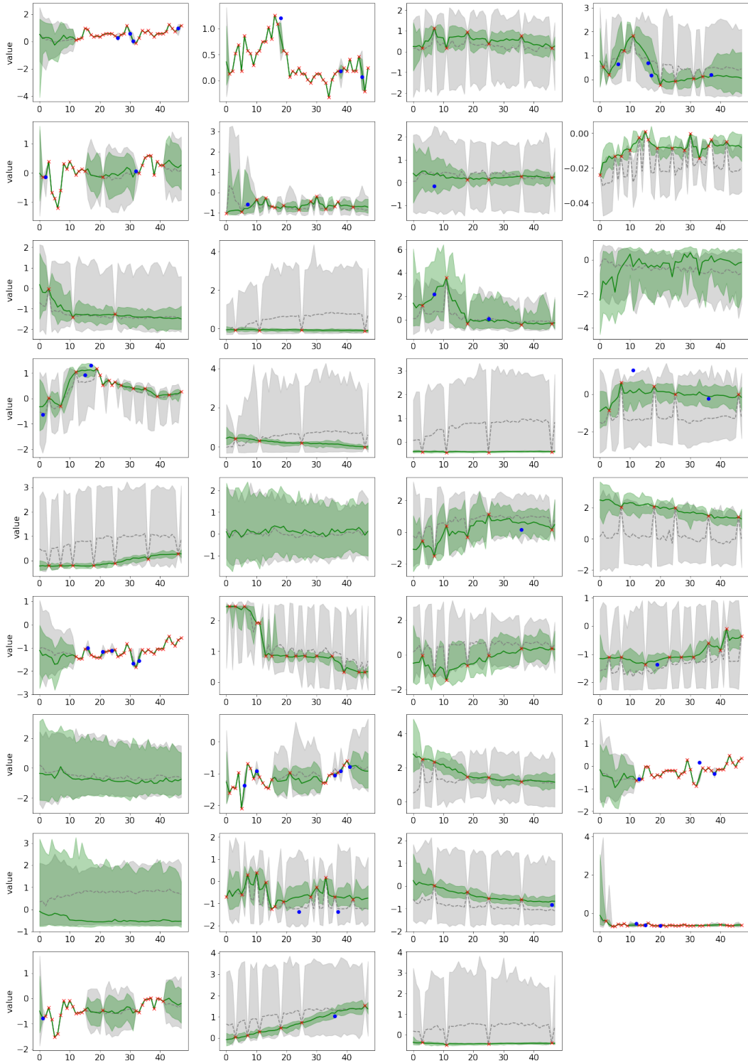
Figure 12: Comparison of imputation between the unconditional diffusion model and CSDI for the healthcare dataset (10% missing). The result is for a time series sample with all 35 features. The red crosses show observed values and the blue circles show ground-truth imputation targets. Green and gray colors correspond to CSDI and the unconditional model, respectively. For each method, median values of imputations are shown as the line and 5% and 95% quantiles are shown as the shade.
