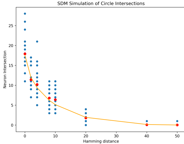
Figure 11: The size of the circle intersection for two vectors at different Hamming distances using simulations vs expectations from Eq. 2 for SDM. We ran 20 simulations with random initialization of all vectors each time for all neuron and pattern addresses. We randomly generated two addresses d_v Hamming distance apart and computed the neuron intersection. Each simulation is a blue dot, the red dot is the mean, and the orange line is the analytical expectation from Eq. 2. For faster simulations, we set n = 100 , r = 10,000 , m = 100 and used Hamming distance d = 35 that activates p = 0.0017 of the space.
