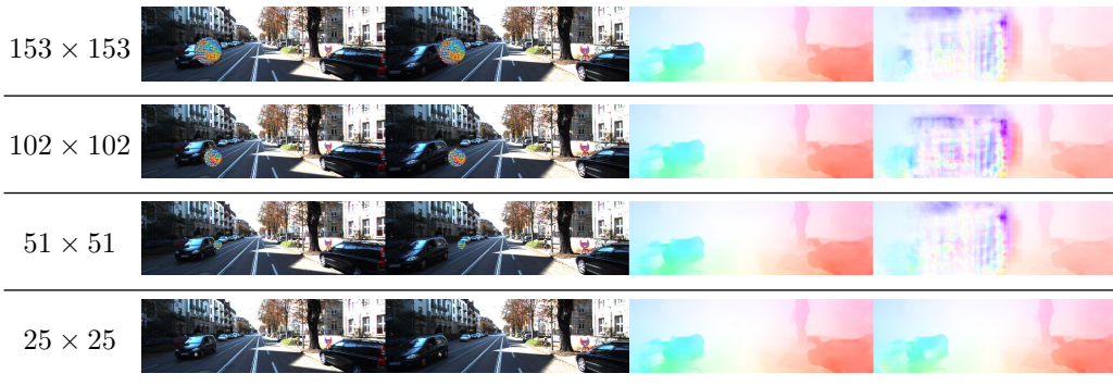
Figure 7: Visualization of the effect of adversarial attack patches on FlowNetC (Dosovitskiy et al. 2015) trained on raw KITTI dataset. In each panel, from left to right: attacked input image 1, attacked input image 2, original estimation of flow, and attacked estimation of flow.
