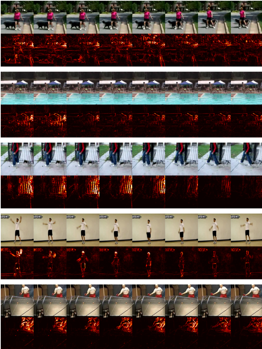
Figure 11: Heatmap of reconstruction errors caused by modifying a single LARP token. The tokens with the same specific index are modified across all 5 videos. In each group, the first row shows the ground truth video frames, while the second row displays the corresponding heatmaps.
