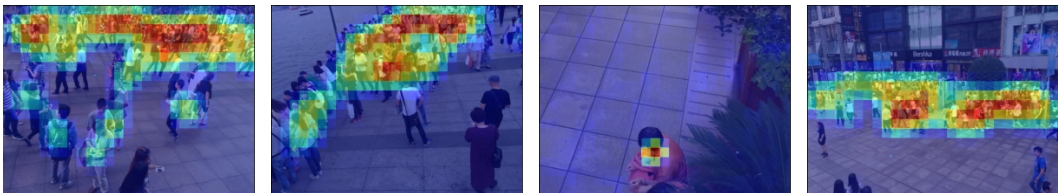
Figure 2: Localization. Heatmap depicting the network’s activation in regions with crowds, derived from features of the last convolutional layer using our method on ShanghaiTechB dataset samples.
