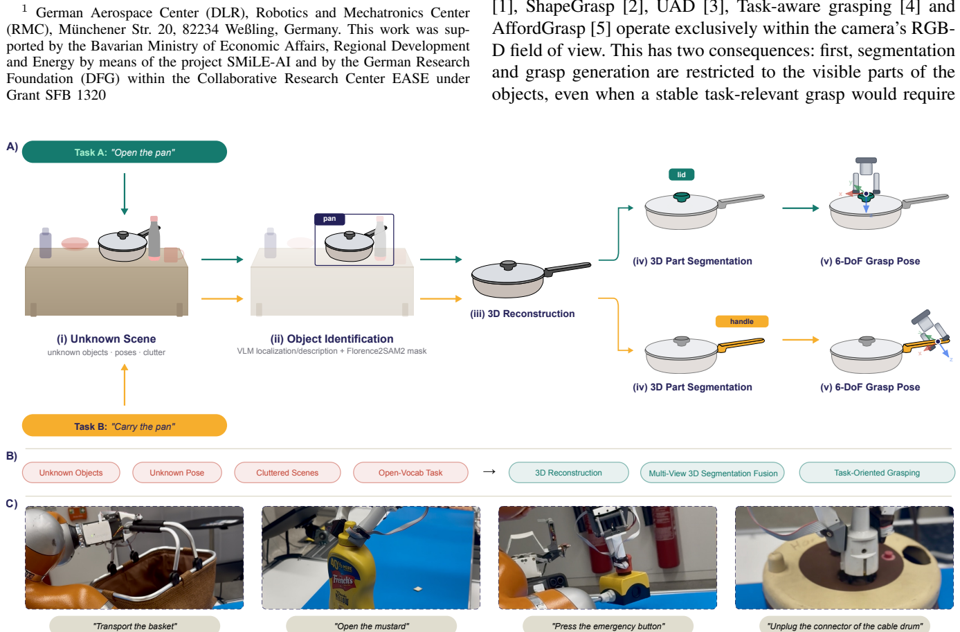
Fig. 1. TIGR pipeline overview. From an RGB-D observation and a natural-language task, TIGR reconstructs the target object, renders it from multiple viewpoints, aggregates part predictions from complementary foundation-model experts into a 3D task-relevant region, and plans collision-aware grasps restricted to that region.
