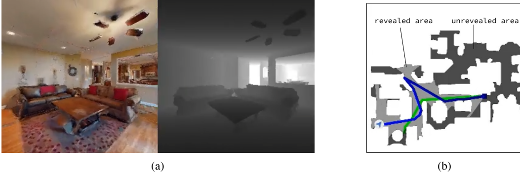
Figure 11: a) Visual observations in Habitat b) Exploration is measured as the proportion of the environment revealed by the agent’s line of sight over the course of the episode.
