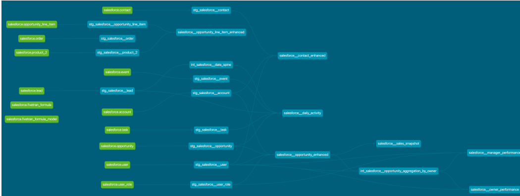
Figure 9: A DAG (Directed Acyclic Graph) illustrating the data flow and dependencies between various Salesforce tables and models in a dbt (data build tool) project. The graph shows stages of transformation, from raw Salesforce data (green nodes) to enhanced and aggregated models (blue nodes), representing different entities such as opportunities, contacts, accounts, and events.
