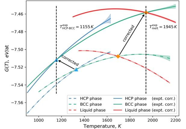
Fig. 3: Free energies of HCP, BCC and liquid phases of Titanium system. Free energies before experimental correction are shown as dashed lines, while those after correction are represented by solid lines. Phase transition temperatures for HCP-BCC and BCC-liquid after correction coincide with experimental values  $T_{\text{HCP-BCC}}^{\text{exp}} = 1155\text{K}$  and  $T_{\text{melt}}^{\text{exp}} = 1941\text{K}$ .
