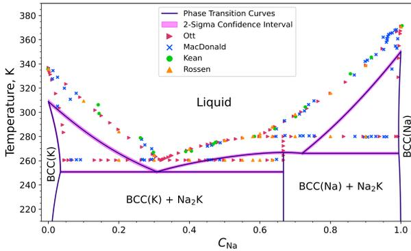
Fig. 2: K–Na phase diagram with a two-sigma confidence interval extrapolated for  $N \rightarrow \infty$ . Experimental data are taken from Ott [4], MacDonald [5], Kean [6], and Rossen [7]. Most features of the phase diagram quantitatively agree with experimental studies, although the resulting phase transition curves are shifted by nearly 20K.
