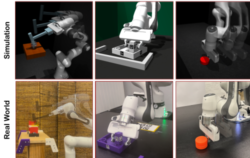
Figure 3: Sim-to-Real Setup Simulation setup for pre-training ( top ) and execution of real-world fine-tuning ( bottom ) of real-world hammering ( left ), insertion ( middle ), and pushing ( right ).
