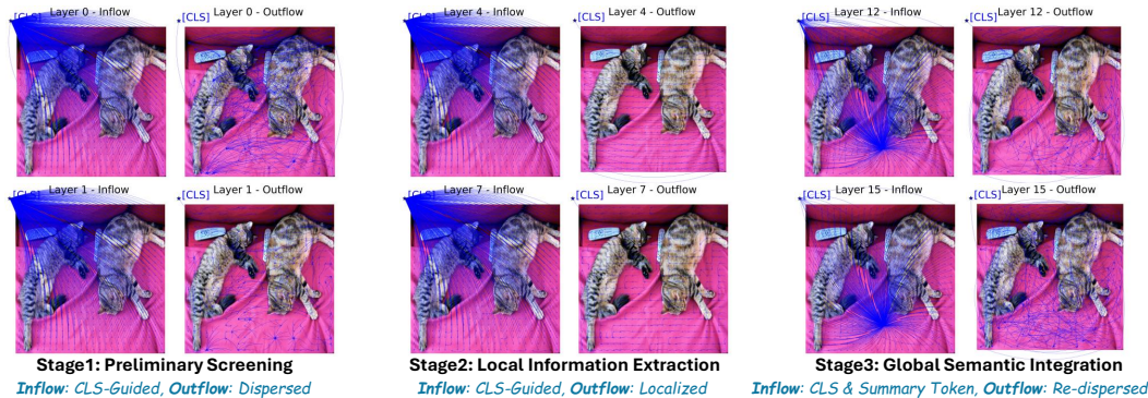
Figure 3: Information flow across different layers of the vision encoder. According to the flows, we can divide the information processing to three stages as Table 1. In stage 3, a token with high attention no longer represents its own local visual content, but instead transforms into a high-level ‘summary token’ Liu et al. (2025); Li et al. (2023c) responsible for integrating global information.
