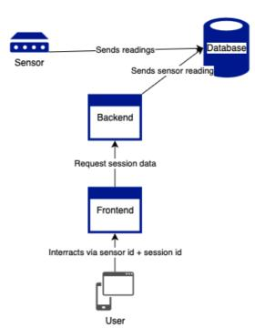
Original idea was to host the application online to allow multiple sensors. This would've required the application logic to be a bit different, as we would need the sensors to send their readings to backend instead of straight to database. We also hostel the model directly in the backend, unlike the we planned originally. Original architecture plan below:
