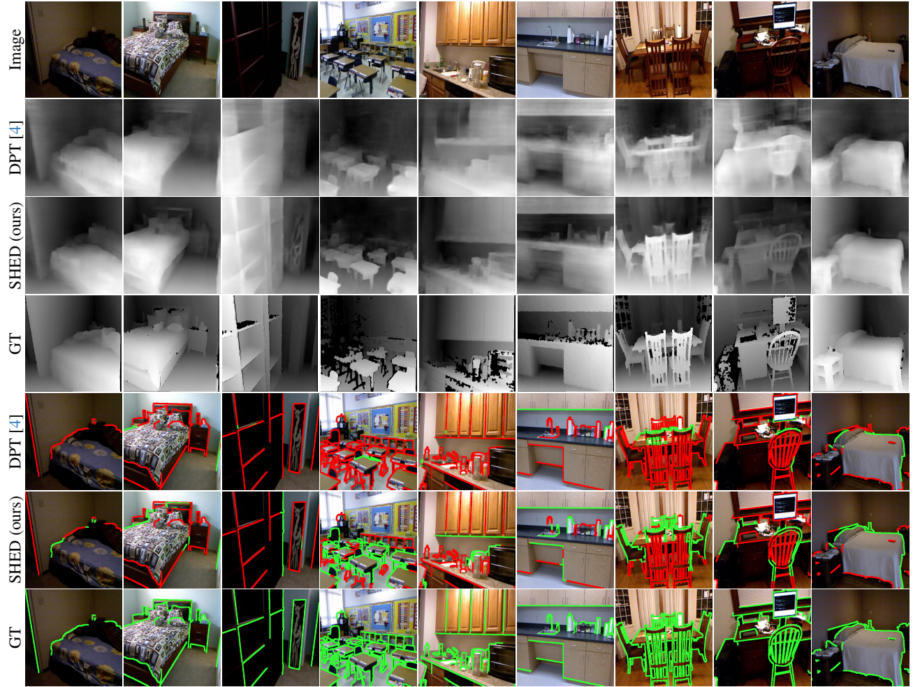
Figure 3. Comparison of depth maps and boundaries. SHED captures more accurate shapes with sharper boundaries, whereas DPT produces blurrier results. As a result, SHED correctly identifies boundaries (green), while DPT fails to detect them (red).
