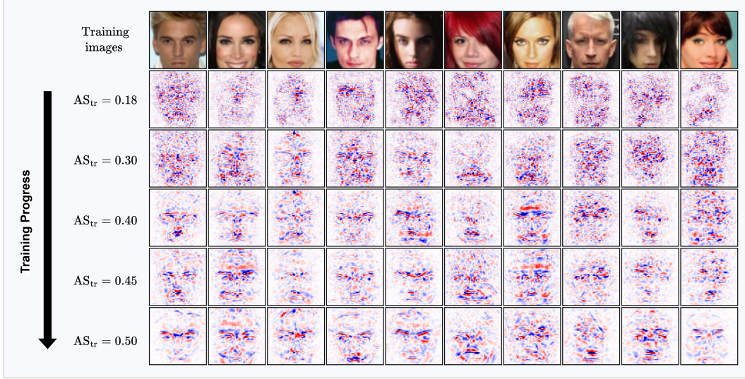
Figure 9: Training-time alignment progression with alignment-aware training. Evolution of training-time alignment score ( AS_{tr} ) and gradient visualizations during fine-tuning of FaceNet using our alignment-aware objective. As alignment improves, loss gradients exhibit increasingly structured and semantically meaningful patterns. (Best viewed with zoom.)
