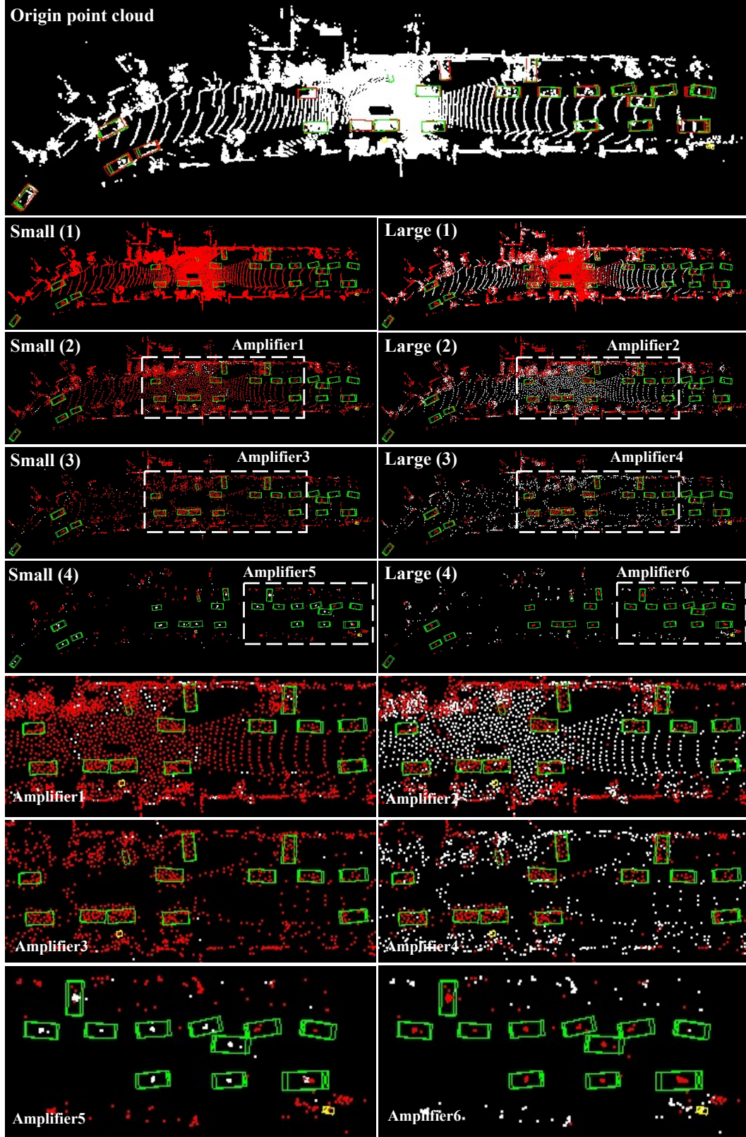
Figure 1: Visualization results on Waymo val set. The red and green 3D boxes in figures are ground truth and prediction boxes. Green, cyan, and yellow represent Car , Pedestrian , and Cyclist . Red and white points represent activation and blocking points, respectively. "Small" and "Large" means the scale of group in MSG, and the digital in parentheses is the index of SA layer.
