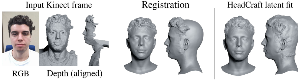
Figure 6. An example of the use case for the HeadCraft registration and fitting stages to Kinect depth data. An example of a frontal RGB frame is shown on the left (the color information is not used further), along with the observed Kinect depth, converted into a mesh and aligned with the standard FLAME coordinate system. We fit FLAME and apply the partial registration procedure, described in Sec. 2, to register the displacements in the observed region (middle) and further fit the HeadCraft latent representation to the corresponding part of the UV map.
